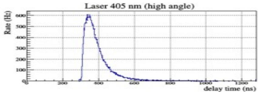
**Figure 2** Photon arrival time distributions as detected from a PMT in the second deployment ( $\sim 15$  m OM distances)
