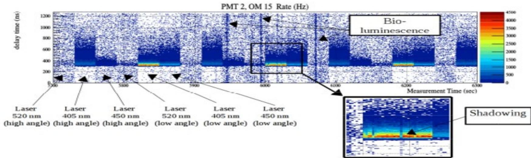
**Figure 3** Part (600 sec) of the "measurement history" as recorded from PMT 2 at the second deployment. In x is the real time of the measurement in seconds; in y are the time channels in the 1280 ns "time window" and in z the hit rate in Hz for each measurement second at each time channel. The 30 sec operation cycles of each laser as well as bioluminescence and shadowing due to life activity can be observed.
