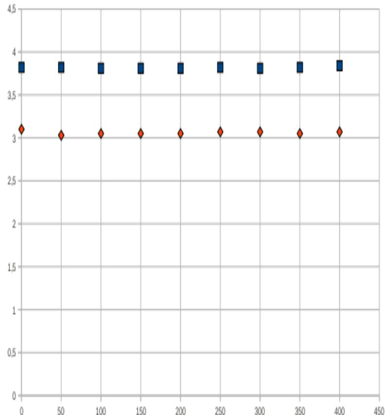
Figure 2 Maximum voltage of the input (blue colour) and output (red colour) signal for each pressure value under test.
