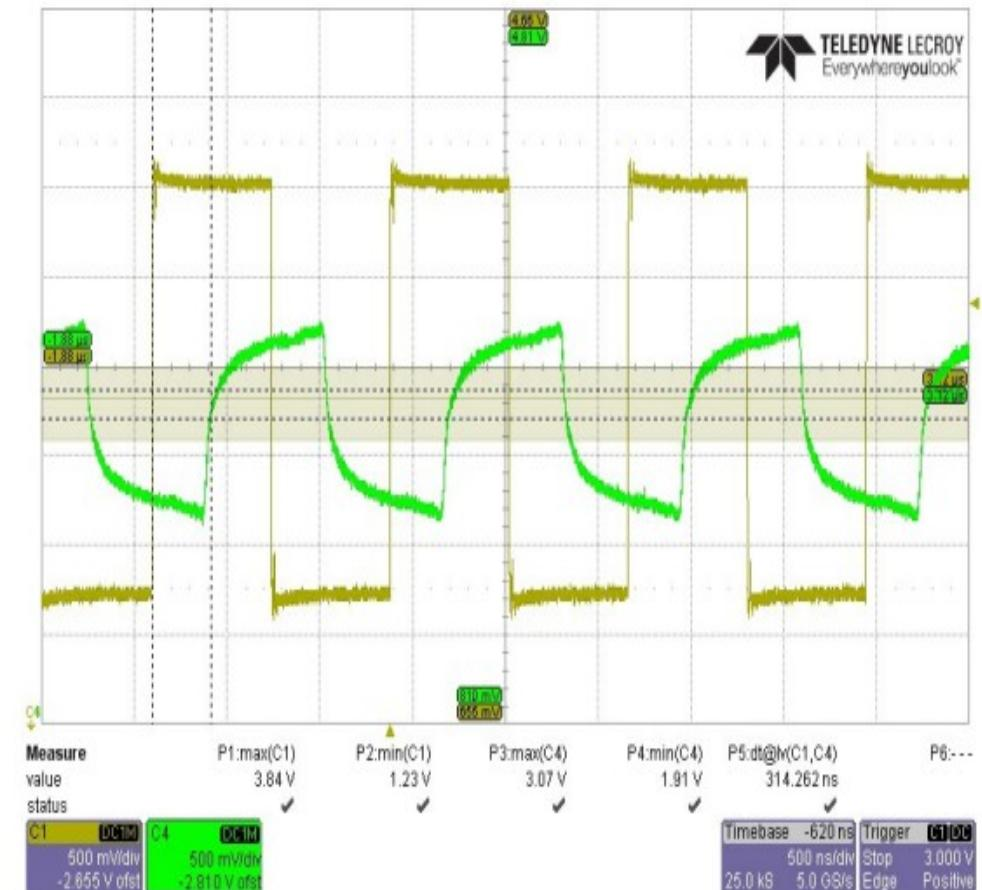
Figure I1 Original signal of 3,84 V that fed the oscilloscope directly (yellow colour) and the signal the came out from the underwater cable (green colour) at 400 bar.
