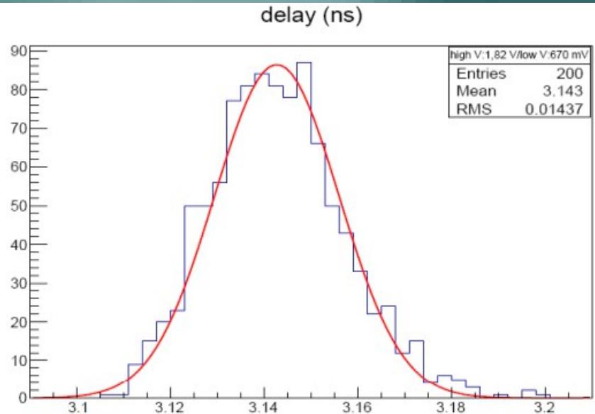
Figure I2 The delay (in ns) of the signal, as measured at pressure 400 bar, fitted to a Gaussian function.
